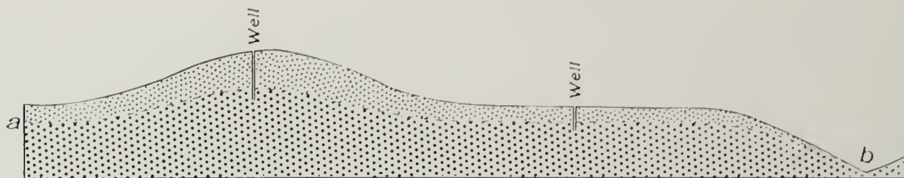
FIG. 24.—Diagram showing the position of the water-table or surface of the groundwater ( a-b ) in a region of undulatory topography and homogeneous materials. The heavily dotted portion is completely saturated.
